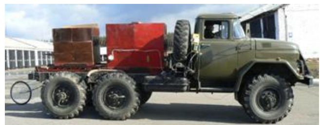
Fig. 6. Truck ZIL-131 with elastically connected elements and set complex of measuring equipment.
