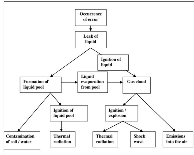
Fig. 1. Consequences of flammable liquid leakage.
