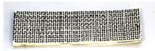
Fig. 2. Microencapsulated halon self-adhesive tape.
