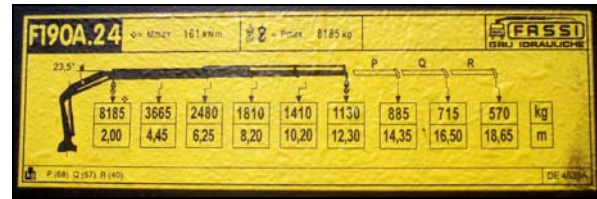
Fig. 11. Working range of rescue automobile (IVECO Trakker) manipulator (F190A.24) depending on the mass lifted
